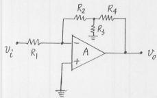
If A is an ideal OP AMP, the voltage gain  $v_o/v_i$  is:
