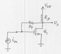
For this circuit with a current source input, the input resistance "seen" by the source is (neglecting  $r_0$  of  $Q_1$ ) approximately:
