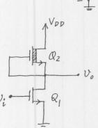
For the circuit in which Q<sub>2</sub> is a depletion mode NMOSFET with Vo<0, which of the operation modes is impossible:
