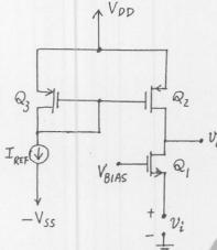
The low frequency small signal gain of this CG amplifier can be expressed as  $vo/vi=(X+r_{01}^{-1})Y$ , where
