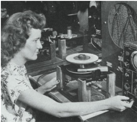
1 Maximum performance of the 45-rpm record player is assured by testing its operation with a sensitive oscilloscope.
